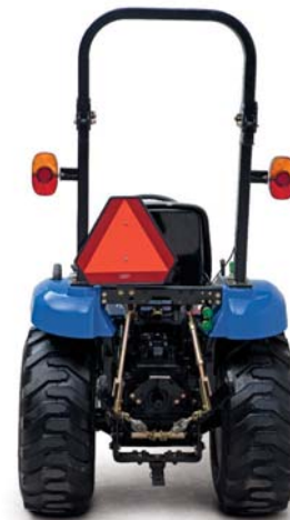
Rear PTO and 3-point hitch allow you to attach countless implements to any job.
