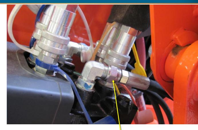
Follow hose to loader valve and remove it from elbow fitting
