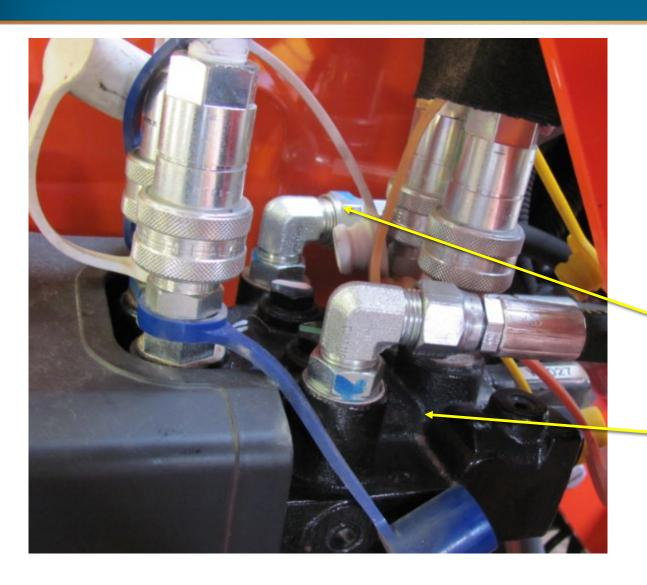
Hose PN# 841-331C will attach to T Port of Valve and other end will connect to loader valve elbow fitting.
