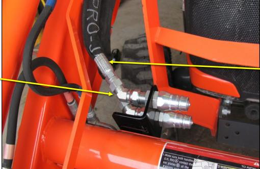
Attach 2 (851-376C) **86"** shielded hoses to JIC side. Run other end of hoses to valve.
