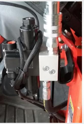
Half inch longer bolts are needed for valve bracket which are not included in kit.
